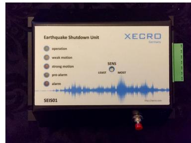
**Sensor:** Dual axis micro-machined polysilicon accelerometers
